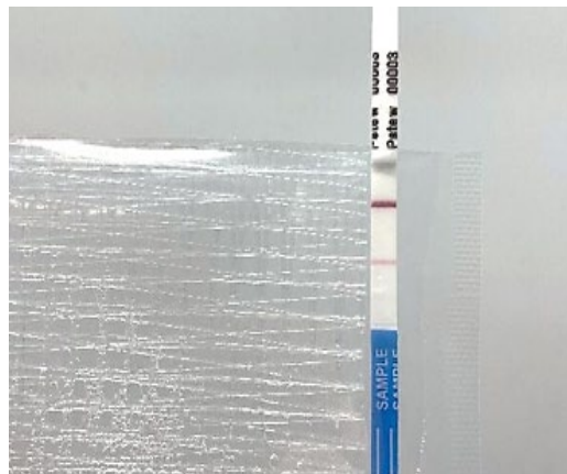
Figure 4. Positive result signified by presence of control and test lines.
