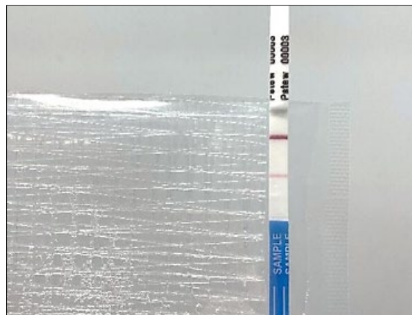
Figure 2. Development of control line (upper) and test line (lower) on ImmunoStrip® in a positive sample.
